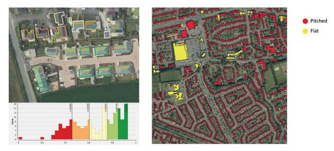
Left: Results from the roof face estimation algorithm. The individual roof faces are shown shaded by their aspect (e.g. yellow is North, dark purple is East). The outline of each building is coloured by how accurate the algorithms results are - these are summarised for the whole test region in the histogram underneath. Right: Results of the flat vs pitch (not-flat) algorithm for a district of Newcastle.
